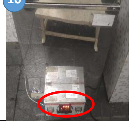
Digital temperature regulator and auto cut off to maintain optimal temperatures to prevent burns
