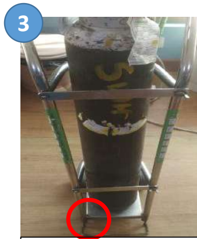
Extended the base of O2 trolley to prevent accidental fall
