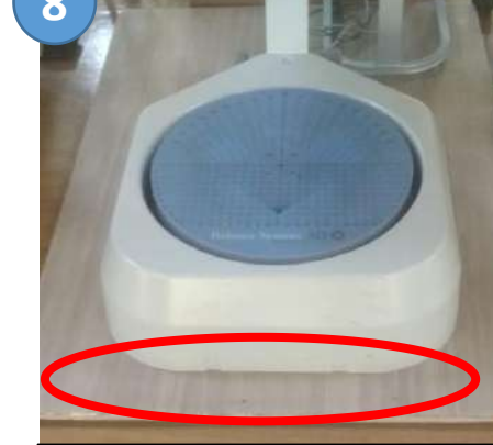
Wooden platform to prevent water seepage and avoid short circuit in Biodex
