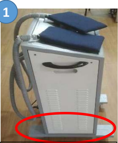
Fixed the base of the SWD unit with a trolley to prevent machine fall
