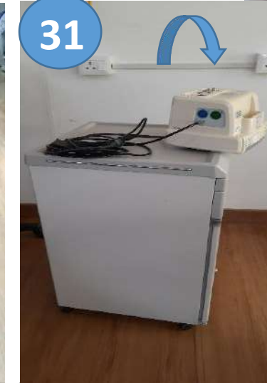
Fabrication of extra base extension for Cardiac monitors for good stability and avoid accidental fall and damage
