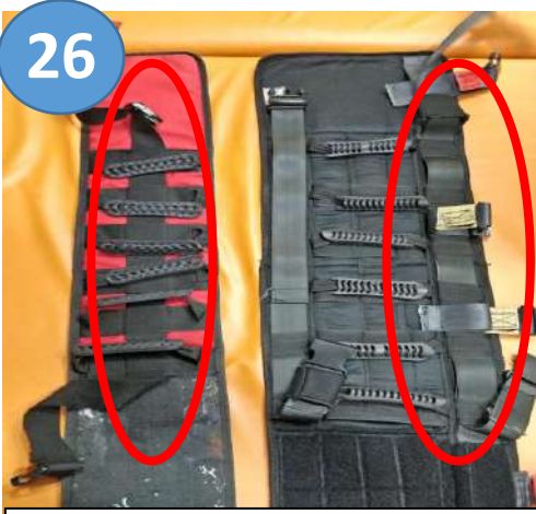
Design and created transfer belts to reduce patient fall during treatment/transfers
