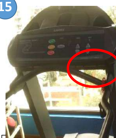
After use the safety switch is removed from the treadmill to avoid sudden start & potential fall
