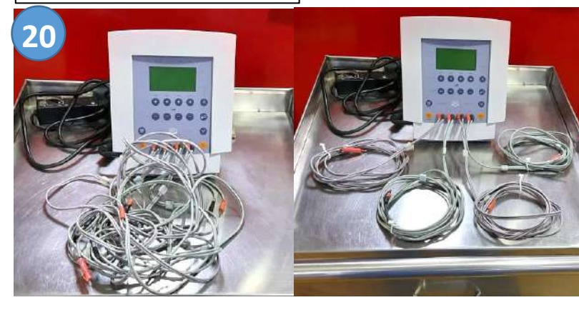
Entangled cables cause damage and cost for replacements.
