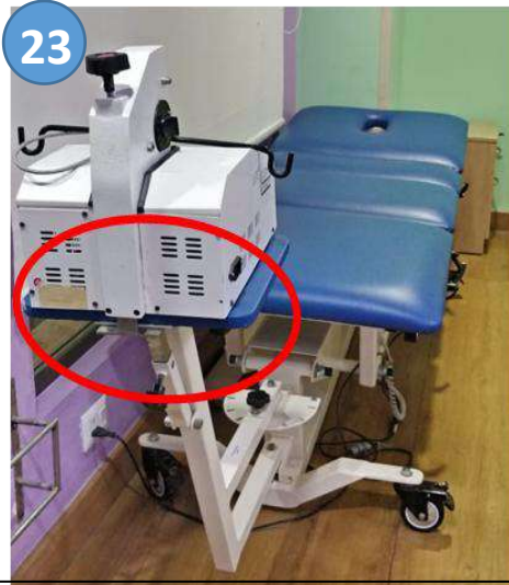
Fixation of traction unit to the base to prevent dislodging and sentinel events
